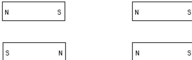
The magnets shown in the left pair are the same distance apart as the magnets in the right pair. In the pair on the left, however, the opposite poles are close together while the similar poles are relatively far apart. The situation is reversed in the other pair. In one case, one would expect the magnets to attract, in the other to repel.
